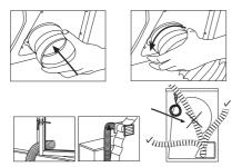
A The air ventilation hose should not be connected to the chimney of a stove or a fireplace.
